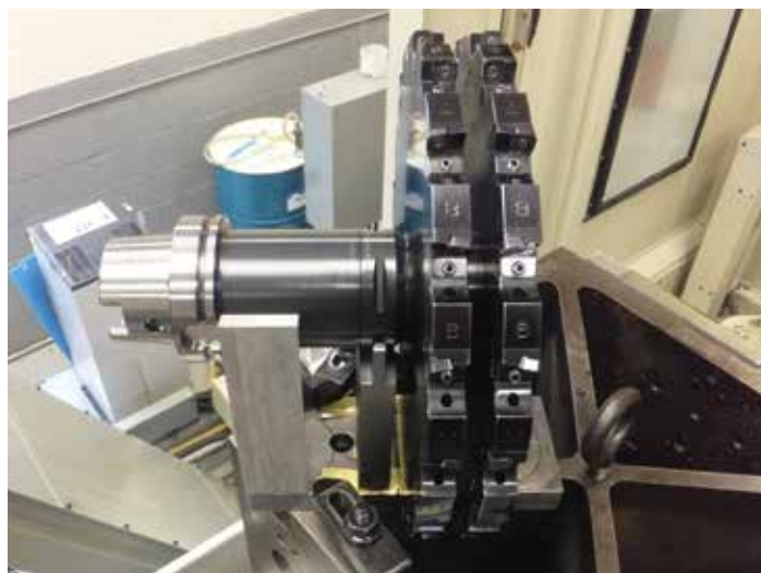
Shop foreman Walter Dzikowski checks the workholding tombstone, which features an in-house-designed and fabricated tool mounting station for a 50-lb custom milling tool. This tool, shown below in the mounting station, has twin slotting cutters that are 13 inches in diameter.
